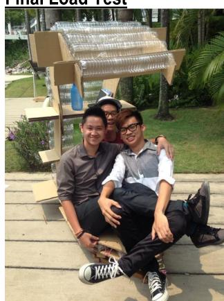
On the day of the testing, a total dead load of 187kg was impacted on the structure. The structure managed to withstand this amount of load for more than 2 minutes, thus, achieving the project goal.
